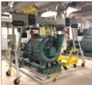
Low headroom 5 tonne Gantry servicing compressors at water plant
